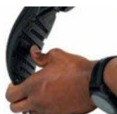
This is printed in a combination of flexible black elastomer and rigid white plastic.
